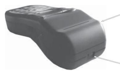
Insert a new printer paper roll as shown in the picture.
