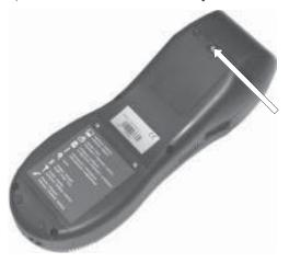
3) Remove the battery pack connector and replace the battery pack  $\,$ with a new one, reversing the operations described above.
