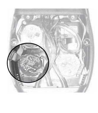
Fig. 5: Example of rotated sensor
